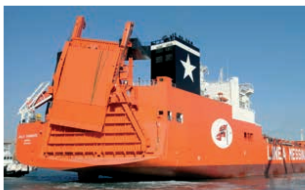
The 50m-long jumbo stern quarter ramp can accept heavy loads on multi-axle trailers and can handle and load containers, breakbulk and project cargo up to seven metres high.
