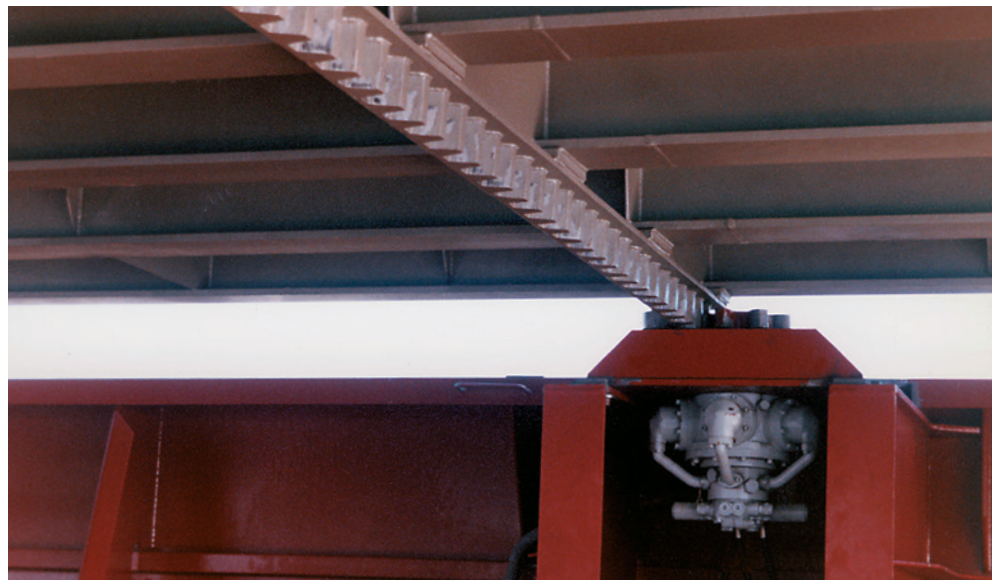
Below: The lifting/securing device of the patented Auto Roll mechanism, with its hydraulic cylinder, wheels and wheel recess, and the auto-cleat device at the ship's centre line.
